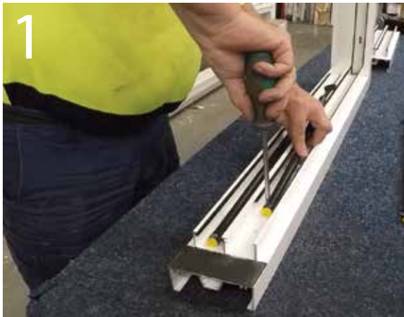
1. Screw springs into jamb (see page 32 for spring placement)
